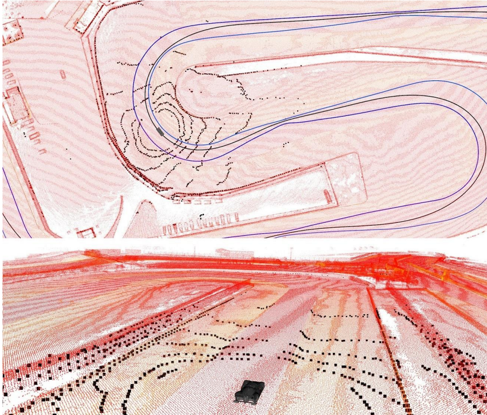
Figure 8: The point cloud map (red) is used to match live measurements (black) that allow to obtain the precise location on the racetrack.
