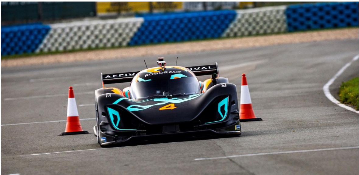
Figure 2: The fully electric ROBORACE DevBot 2.0 passes a gate on the Circuit de Croix-en-Ternois in France [13]. The Ouster OS1-16 LiDAR [14] for localization is placed on the top of the race car.
